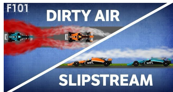
Figure 6 - dirty air versus slipstream
